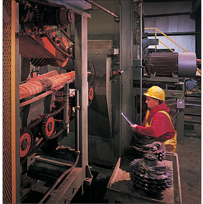
A Baldor•Reliance 500 Hp, medium voltage Severe Duty Motor (pictured at the back end of the machine) and Series 22H Line Regen Vector Control run this chipping machine at a North Carolina lumber mill. High performance and reliability are the hallmarks of this Baldor motor, running in multiple shifts, under high-torque demands, exposed to sawdust and other airborne contaminants.
